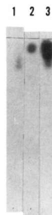
Figure 6. TLC analysis of the radioactivity collected from Dowex AG 1X8 resin column. (Lane 1) Authentic selenocysteine; (lane 2) authentic selenomethionine; (lane 3) radioactive pool from Dowex AG 1X8 column when the purified SRP 6 N HCl hydrolyzate was fractionated. Direction of migration is from bottom to top (ascending TLC).
